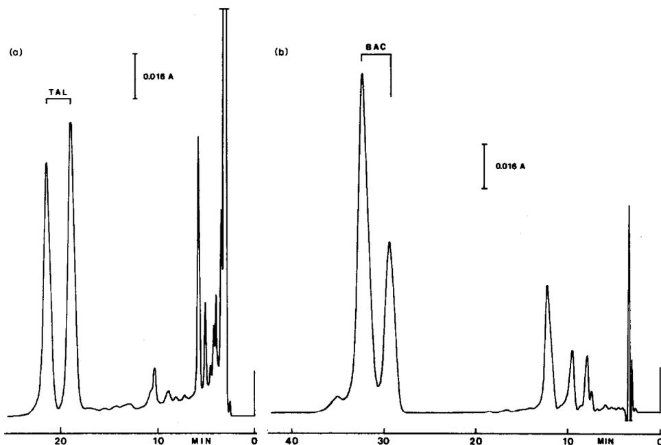
Fig. 2. High-performance liquid chromatograms of (a) talampicillin hydrochloride and (b) bacampicillin hydrochloride on Zorbax  $C_8$  (25 cm  $\times$  0.46 cm) with ethanol-water-0.2 M phosphate buffer pH 7.0 (40:55:5) as the mobile phase. Detection: 254 nm, 0.16 a.u.f.s. Amount injected: 100  $\mu$ g. Old samples were chosen to demonstrate the selectivity of the chromatographic system.
